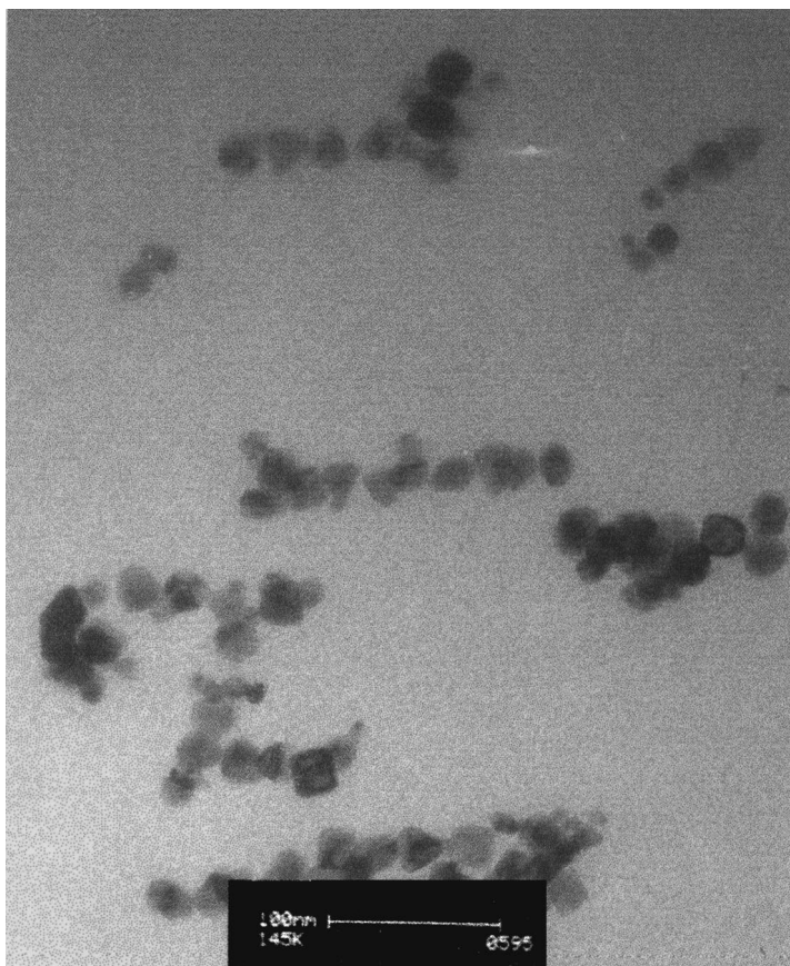
Fig. 2. TEM micrograph of Pd nanoparticles stabilised by microgel M1.
